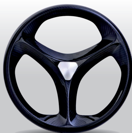
Keywest PC 25482N Polished carbon fiber and TPU grip and spokes.
