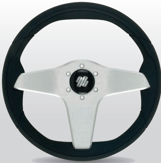
CAPRAIA B/S 22958X Ø 350 mm (13.8") Depth 84mm (3.3") Black polyurethane grip, silver aluminum spokes
